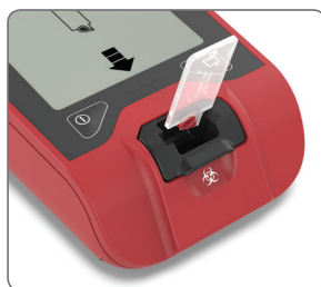
2 Place microcuvette into analyzer.
